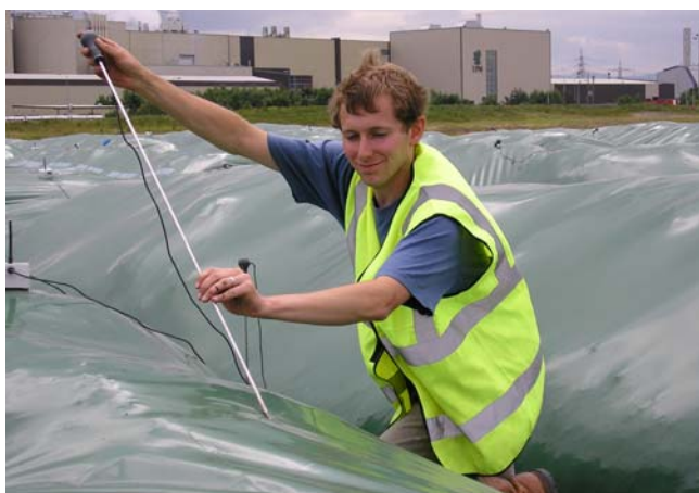
A 1 m long probe records temperature at the surface and centre of the EcoPOD®
